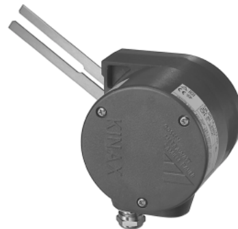
Fig. 2. Position feedback transmitter KINAX SR 719 showing the operating lever in the upper zero position, corresponding output current 4 mA.
