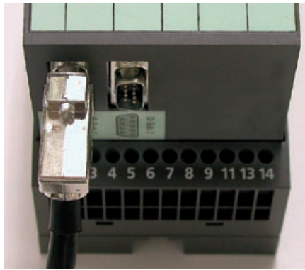
2 plug connectors (9-pin D-SUB) each for 3 low voltage signals from electronic current and voltage transformers.
